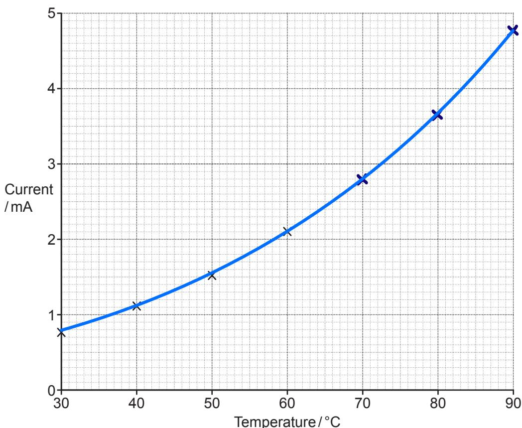
(c) Describe, using the graph and calculations using data from the table, how the resistance of the thermistor varies for increasing temperature.
