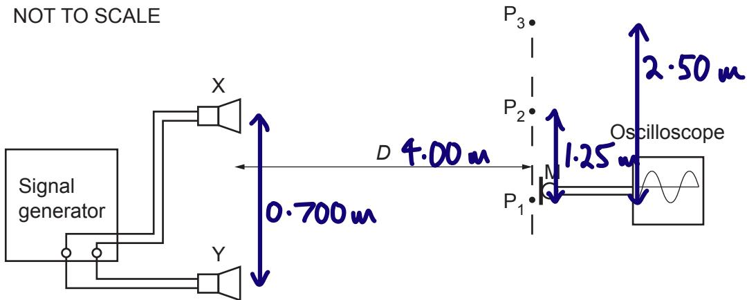
As the microphone is moved along the line  $P_1$  to  $P_3$  the oscilloscope shows maximum signal at  $P_1$ , zero signal at  $P_2$  and the next maximum signal at  $P_3$ .
