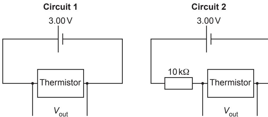
In each circuit, the voltage  $V_{out}$  across the thermistor is connected to the heating system for warming the milk.
