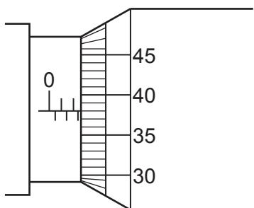
$$\begin{aligned} \text{Take off zero error} \\ A &= \frac{\pi d^2}{4} = \frac{\pi \times (2.81 \times 10^{-3})^2}{4} \\ &= 6.202 \times 10^{-6} \text{ m}^2 \end{aligned}$$
