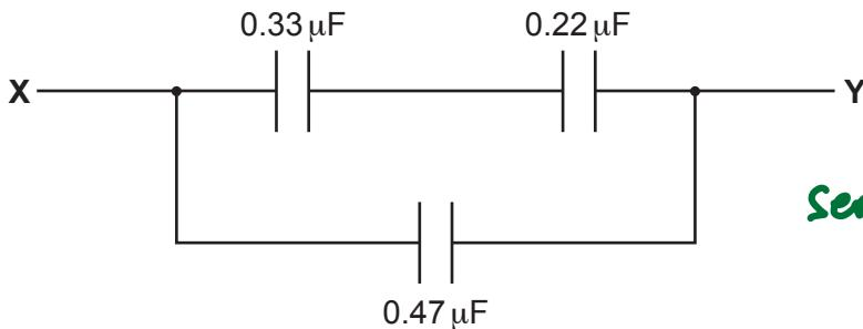
$$\text{series: } \frac{1}{C_T} = \frac{1}{C_1} + \frac{1}{C_2}$$
