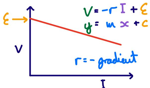
They measure the current and potential difference (p.d.) across the variable resistor for different resistor values.
