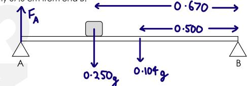
a. Calculate the total **anti-clockwise** moment of the ruler and mass about the point B
