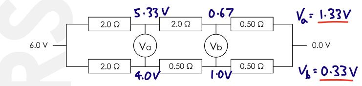
1. Calculate the **reading** on the high-resistance **voltmeters**  $V_a$  and  $V_b$ .
