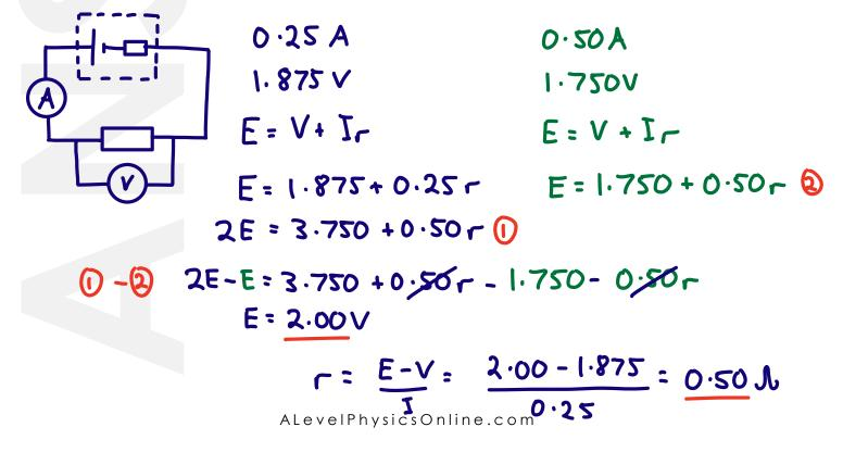
1. A student connects a cell in series with a variable resistor and an ammeter. They connect a voltmeter in parallel with the cell. They alter the value of the variable resistor and obtain the results below.
