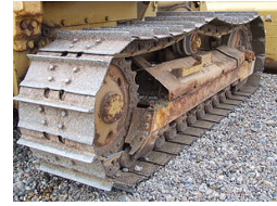
Figure 6: The moving caterpillar track on a bulldozer.
