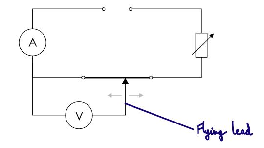
An alternative approach to measure resistivity is with the following circuit:
