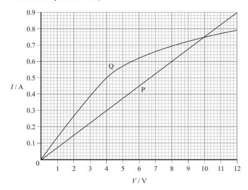
(i) State the value of the current for which the resistance of P is the same as the resistance of Q and determine this value of resistance.
