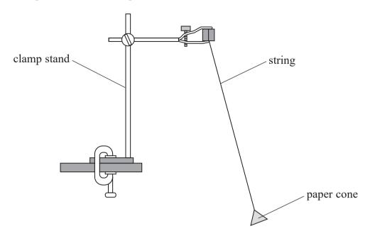
(a) (i) The student displaced the pendulum through a small angle so that it oscillated. She determined the time period T as  $2.50 \,\mathrm{s}$ .
