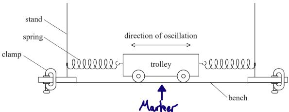
The student displaced the trolley from its equilibrium position. She then released the trolley and started a stopwatch. She stopped the stopwatch when the trolley had completed one oscillation.
