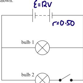
Each bulb has a normal working power of 40 W when a potential difference (p.d.) of 12 V is applied.
