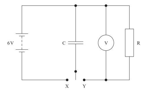
The student used the switch to connect C to X to charge the capacitor. She then connected C to Y to discharge the capacitor through R.
